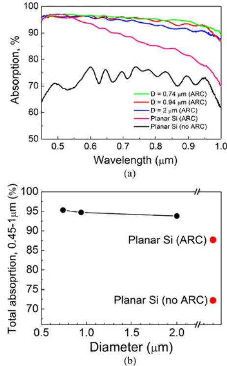
Fig. 4. Absorption spectra (a) and total absorption rate of (b) Si micropillar array based structures of various diameters, as well as the reference planar structures, in the wavelength range from  $0.45$  to  $1\text{ }\mu\text{m}$ .
