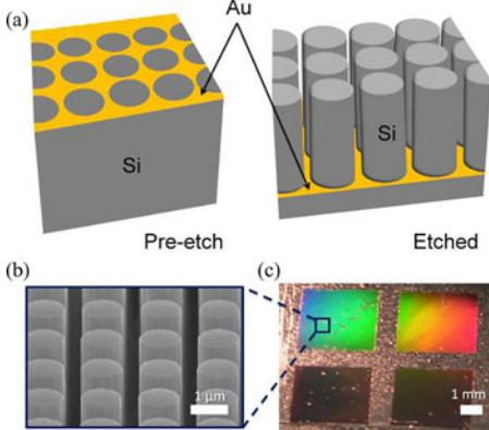
Fig. 1. (a) Schematic illustration of the MacEtch mechanism, where the metal pattern (Au mesh in yellow color) descends by etching Si directly underneath resulting in a 3-D Si structure (Si pillars are in gray color). (b) 45° tilted SEM image of Si micropillar array produced by Au-MacEtch. (c) Optical image of MacEtched micropillar arrays. Each square consists of pillars of different diameters.
