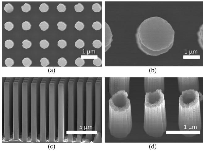
Fig. 3. Top SEM views of the (a) smallest ( $0.54\text{ }\mu\text{m}$ ) and (b) largest ( $2\text{ }\mu\text{m}$ ) diameter pillars used in this study under the same magnification. (c)  $85^\circ$  tilted SEM view of a micropillar array with highly vertical, nontapered sidewalls. (d)  $5^\circ$  tilted SEM view of hollow pillars after selectively removing the p-type cores leaving behind the  $n^+$  cylindrical shells by dipping in KOH solution for 2 s.
