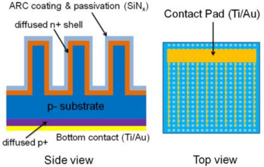
Fig. 2. Schematic illustrations of the solar cell structure, (left) cross section and (right) top view, with the core-shell junction and metal contact scheme indicated. The pillar height and tray thickness are not to scale.
