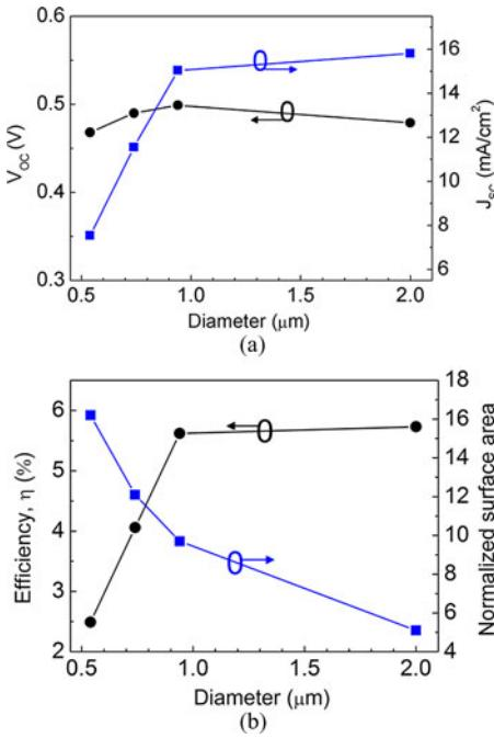
Fig. 6. (a)  $V_{oc}$  and  $J_{sc}$ , and (b)  $\eta$  and top surface area of the micropillar-based solar cells as a function of pillar diameter.
