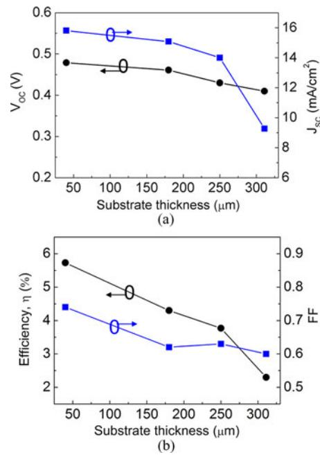
Fig. 5. (a)  $V_{oc}$  and  $J_{sc}$ , and (b)  $\eta$  and FF, of a 2-mm-diameter micropillar array solar cells as a function of Si membrane substrate thickness.
